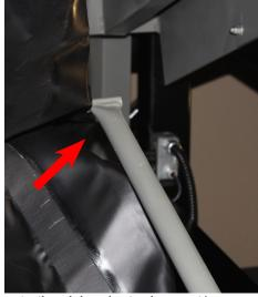
(Left - Bag is off-center and falling off of skid. Right - Maintenance prop is contacting air bag due to placement.)
