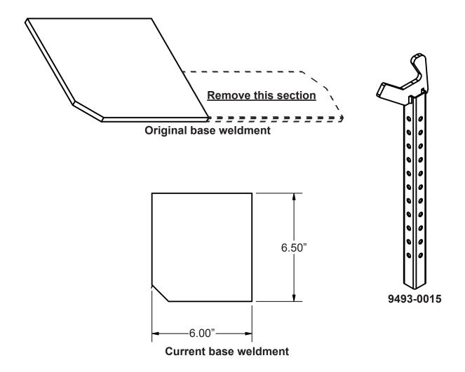
After the original base weldment has been trimmed and the additional catch assembly has been purchased, the Tough Strut can be used on Mechanical, AP, DA, MA and CentraAir units with catch 9493-0007, and on DH, EH, H, HP and VH models with catch 9493-0015.\*
