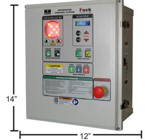
**INSTALLATION:** Requires mounting of locking unit, control panel, exterior lights and signs in strict accordance with DLM<sup>®</sup> installation instructions. TPR can be welded to an optional new construction embed plate or by installing 15 anchor bolts (included) plus 16" of weld to dock curb steel. Mechanical installation is recommended to be performed only by authorized DLM Representative.
