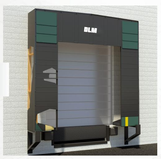
Rigid Series Dock Shelter—provides maximum dock protection and full access to trailers while minimizing pressure on the building wall. The RF Series features high wear-resistant fabric with double lock-stitched seams, bottom corner draft pads, protective corner reinforcement pleats, wind retention straps and a 36-inch drop head curtain with fiberglass stays. The raked header with translucent fiberglass top provides natural light, permits water drainage, and provides snow load support.
