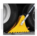
The chock system is installed with an articulated arm and ground plate to lock the chock in position.
