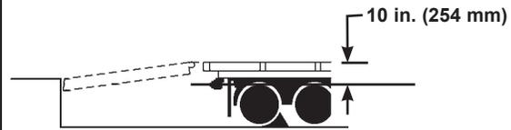
The HSM hydraulic dock leveler is designed to compensate for a maximum + 10 in.\* (254 mm) of height difference between the loading dock and the transport vehicles bed. DO NOT use the dock leveler if the transport vehicles bed is more than 10 in. (254 mm) higher than the dock floor.
