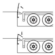
1. Press the RAISE button until the lip folds enough to clear the transport vehicle, then release the RAISE button. The lip will fold and the platform will lower returning to the stored position.
